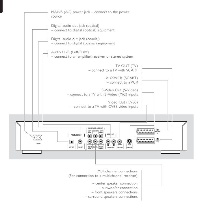
Caution: Do not touch the inner pins of the jacks on the rear panel connectors. Electrostatic discharge may cause permanent damage to the unit.
